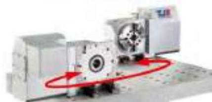
Application diagram: retrofits 3-axis-moving-column vertical machining center with CHC
