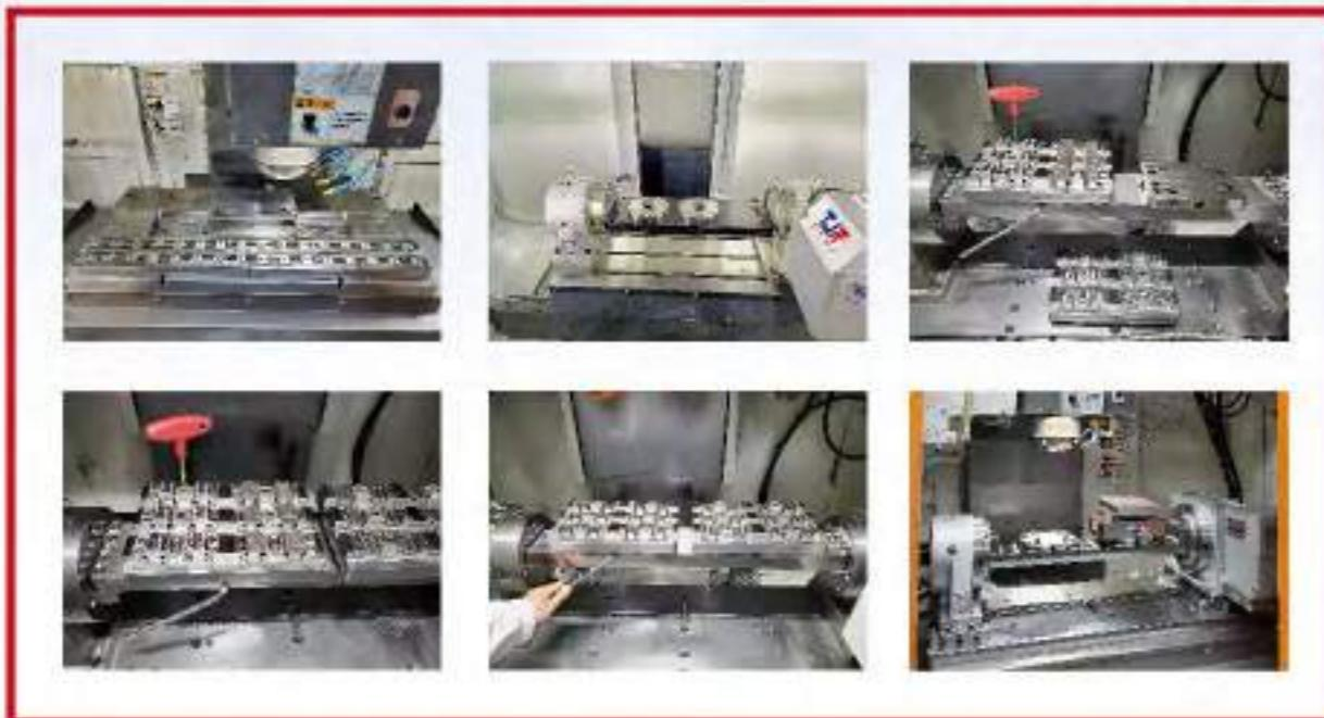
**A built-in zero point clamping system on the faceplate of tilting rotary table.**
